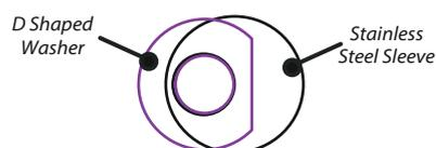
Figure 1 - top view showing how the D shaped washer aligns with the stainless steel sleeve
